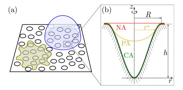
the nanopit, a partially-adhered state (PA) if the membrane only shallowly enters the nanopit, and a completely-adhered state (CA) if the membrane is fully bound to the nanopit and closely follows its shape.
